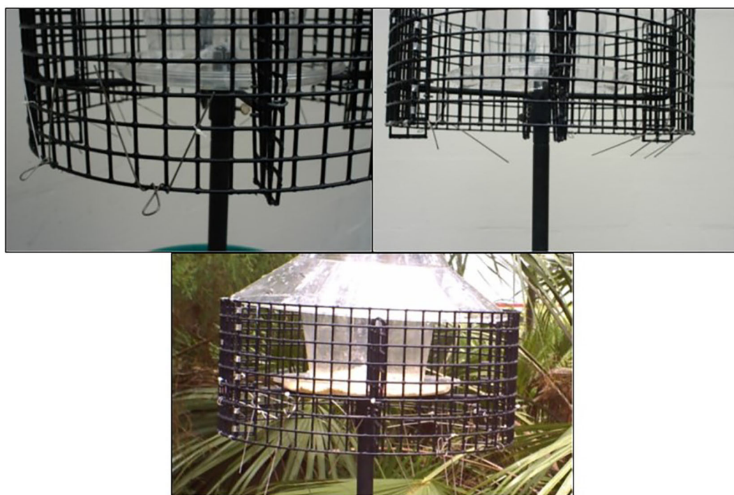
FIGURE 2 Modifications to the parakeet-selective feeder designed to reduce access by nontarget species: stiff wires not deployed (top left), stiff wires deployed (top right), and dangling wires (bottom).
